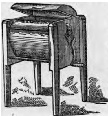
FIG. 22.—The Modern Rotary Churn, Blanchard type.
